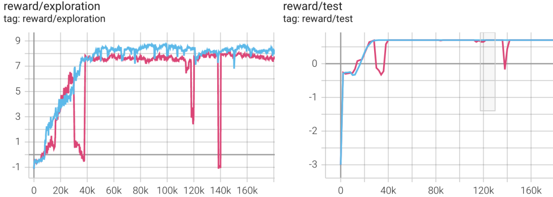
Figure 3: Exploration and exploitation rewards for baseline DREAM (blue) and task-specific exploration DREAM (red) on the basic map grid environment trained for 180k episodes
